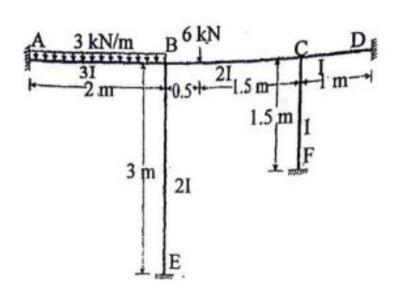
4. (a) A beam ABCD, 15 m long is continuous over three spans and is loaded as shown in Fig. Calculate the moments and reactions at supports by the moment distribution method.
