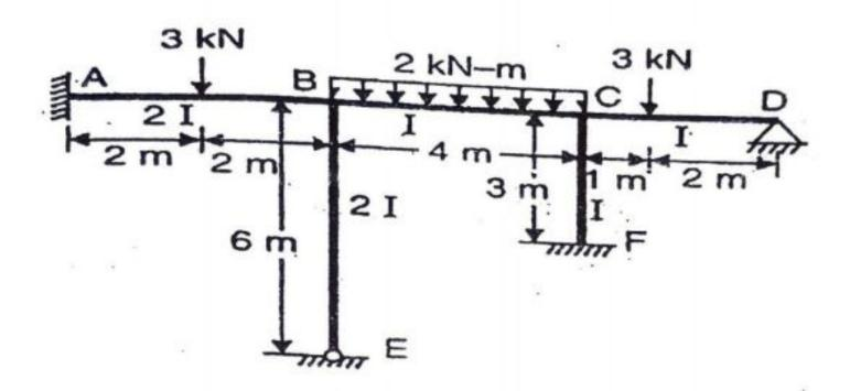
5. A continuous beam ABCD consists of three spans and is loaded as shown in fig. Ends A and D are fixed. Determine the bending moments at supports, using Kani's method. Also plot the bending moment diagram and deflected shape of the beam.
